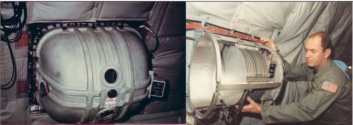
The U-1 foil has been the heart of particulate sampling since 1962. At left is foil in WC-135 with cover installed. At right SEO shows what the record changer mechanism looks like. The U-1 is generally loaded pre-flight and unloaded post-flight by MET/ARE. A foil was only opened in flight if something jammed, which thankfully rarely happened. Photos courtesy of Dennis Goens
