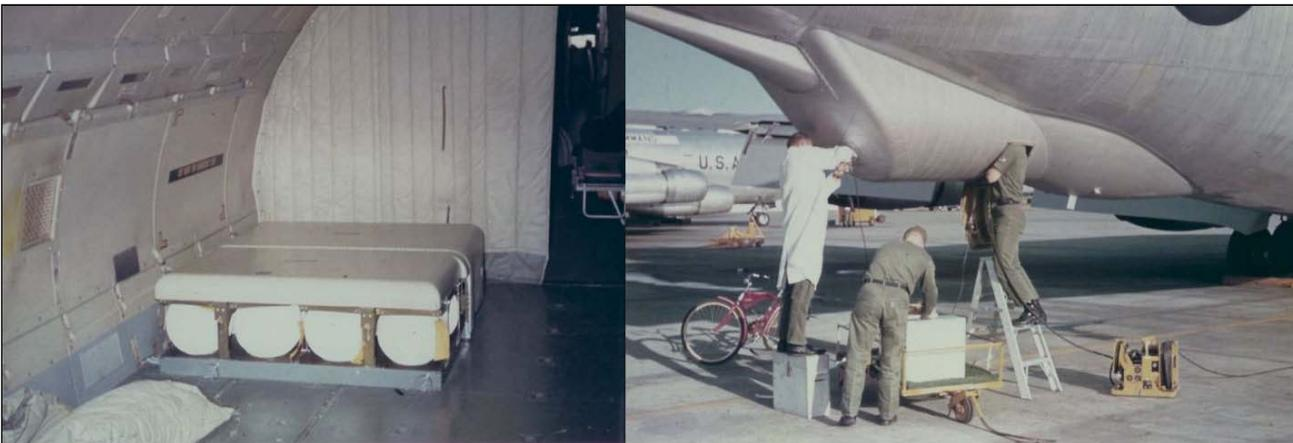
At left is Pressure Platform, or P-System, in WC-135. The P-System allowed crew to gather whole air samples for laboratory analysis. This photo gives some idea of what made the WC-135 such a great platform – room and more room! At right, 3-man MET/ARE team loads the 9-Shot revolver dropsonde system. Similar system used on the WB-47E. Photos courtesy of Dennis Goens
